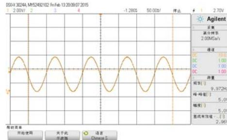
Figure 15: 10Hz sine wave
