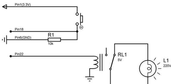
Fig. 3. Light module control circuit
