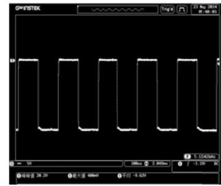
Figure A PWM microcontroller output a wave
