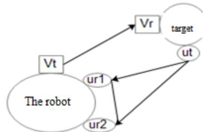
Fig.1 The principle diagram of ultrasonic positioning
