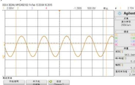
Figure 14: 1Hz sine wave
