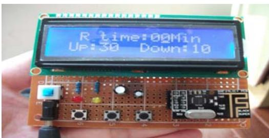
Figure8:Host of the wireless system of testing temperature and humidity.
