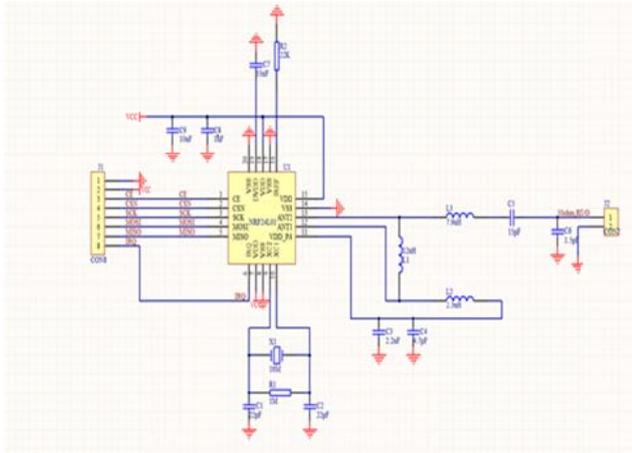
Figure 2: nRF24L01 wireless module circuit diagram
