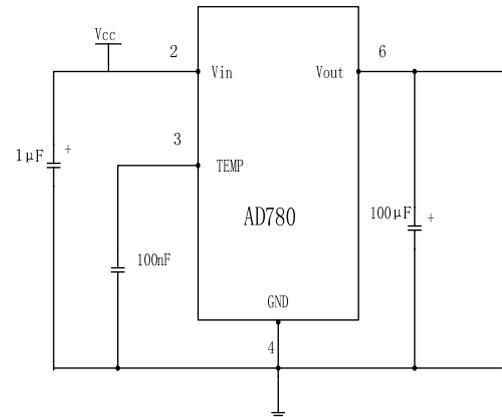
Figure 2 AD780 wiring mode
