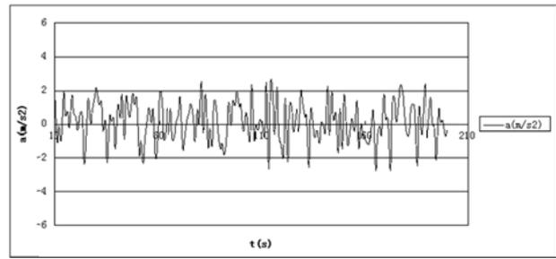
Figure 6. normal walking acceleration curve
