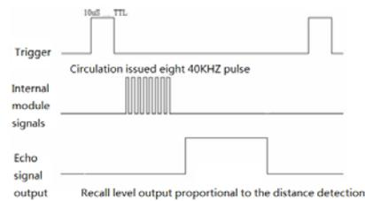
Fig 3 Ultrasonic timing diagram
