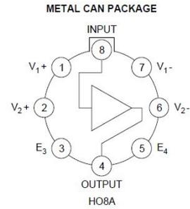
Figure 12: LH0002 pin diagram
