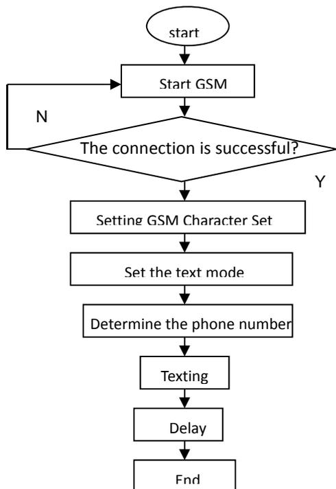
Fig.7 The work flow chart of SIM900A communication modul
