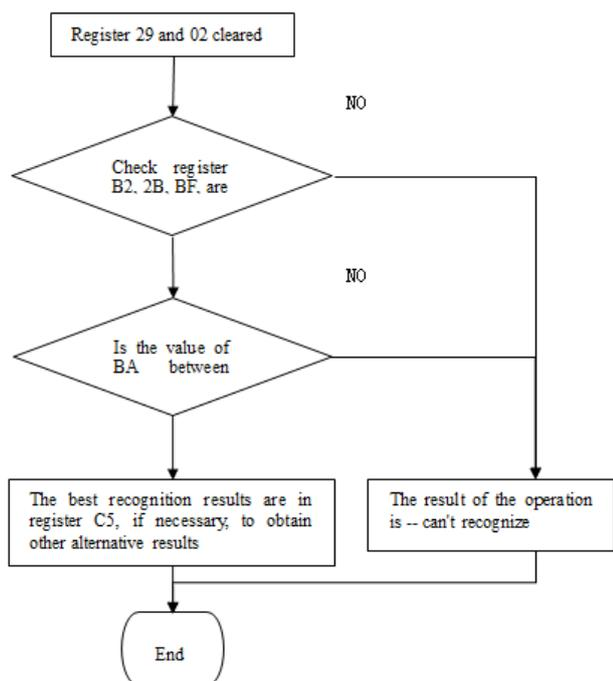
Fig.8 Response interrupt flow chart
