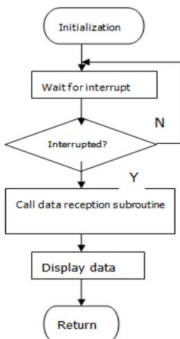
Figure 5: Main flow chart of data receiving and display section.
