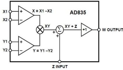
Figure 9: multiplier function block diagram
