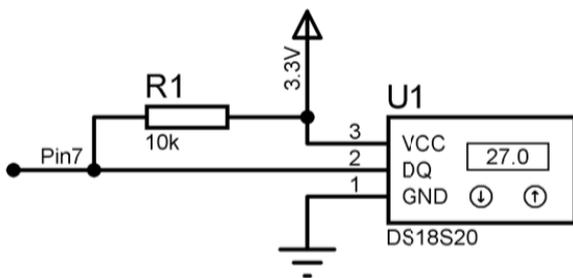
Fig. 7. Temperature Module Circuit
