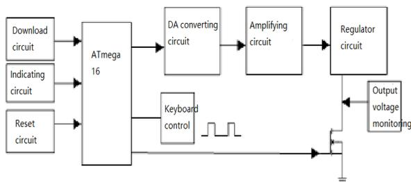
Figure 1 Overall structure diagram
