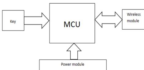
Fig.2.2 search and rescue card system block diagram
