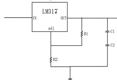
Figure 10 Voltage regulator circuit
