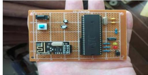
Figure9:Slave of the wireless system of testing temperature and humidity.
