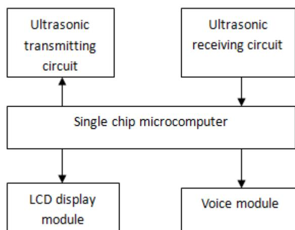
Fig 1 Diagram of the system's structure
