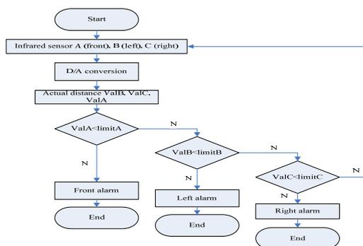
Fig.3.2 Infrared distance sensors in three directions of priority judging flow chart
