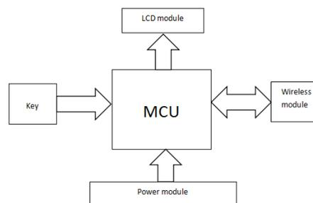
Fig.2.3 block diagram of the search and rescue apparatus
