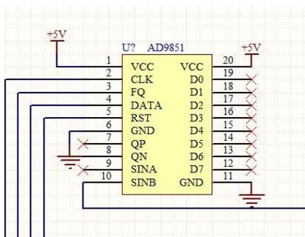
Figure6 : Signal generating module
