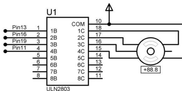
Fig. 5. Stepping motor driving circuit
