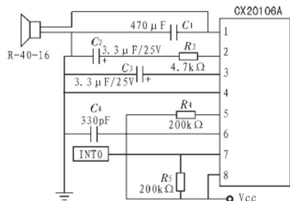
Fig.3 The main circuit of ultrasonic receiving
