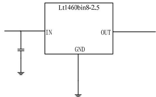
Figure 3 Lt1460bin8-2.5 wiring mode
