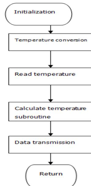
Figure 3: Main program flow chart of data acquisition and emitting
