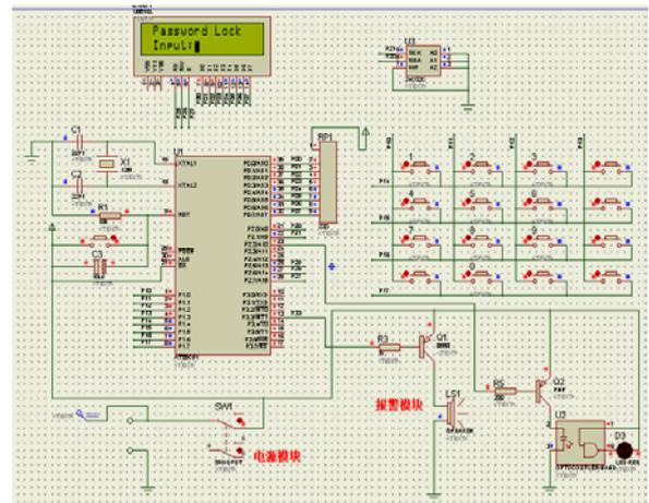
Fig.3 The whole simulation diagram of the Combination lock
