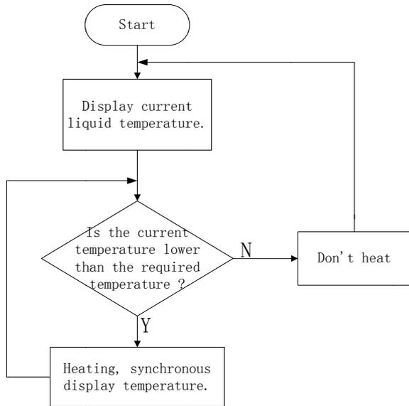
Figure 4. The heating temperature control module flow chart
