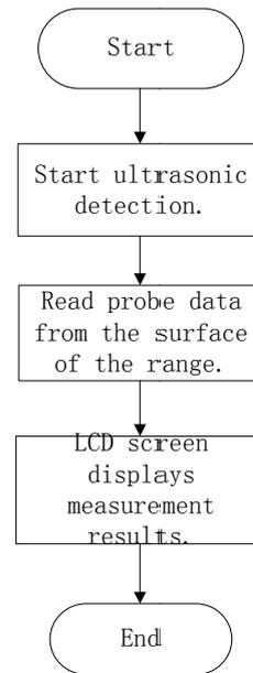
Figure 5. Level module flow chart
