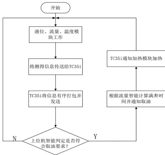
Figure 3. The overall work flow chart
