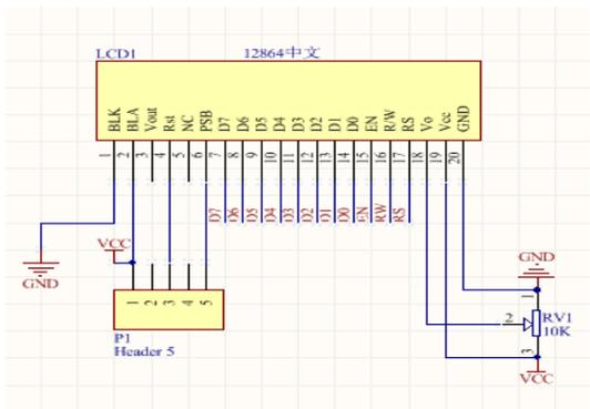
Fig 6 LCD circuit
