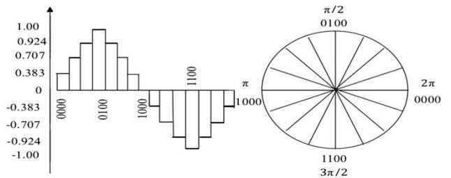
Figure 1:Phase and amplitude map
