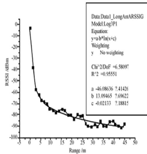
Fig.4.1 RSSI and distance fitting curve
