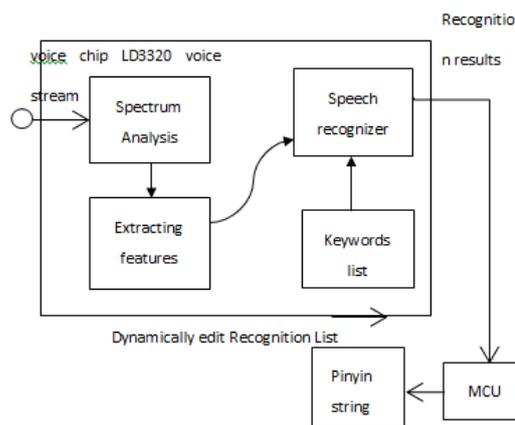
Fig.4 Chip principle block diagram
