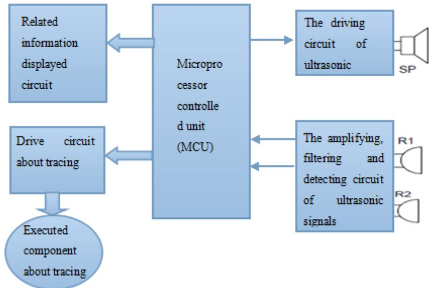
Fig.2 Composition and structure of ultrasonic target positioning system
