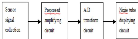
Fig.4 Weighing module workflow
