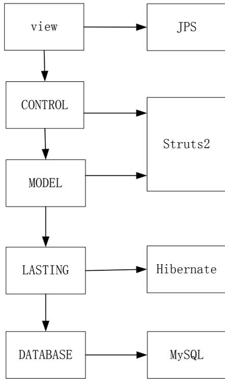
Figure 5. Server architecture diagram
