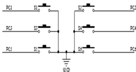
Figure 11 Keyboard circuit
