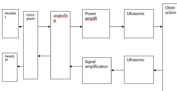
Fig 2 Hardware structure diagram
