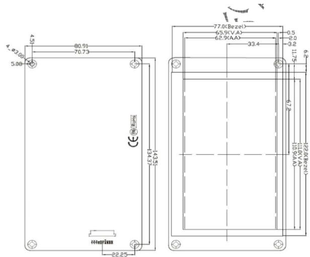
Fig.4 Module machine size chart
