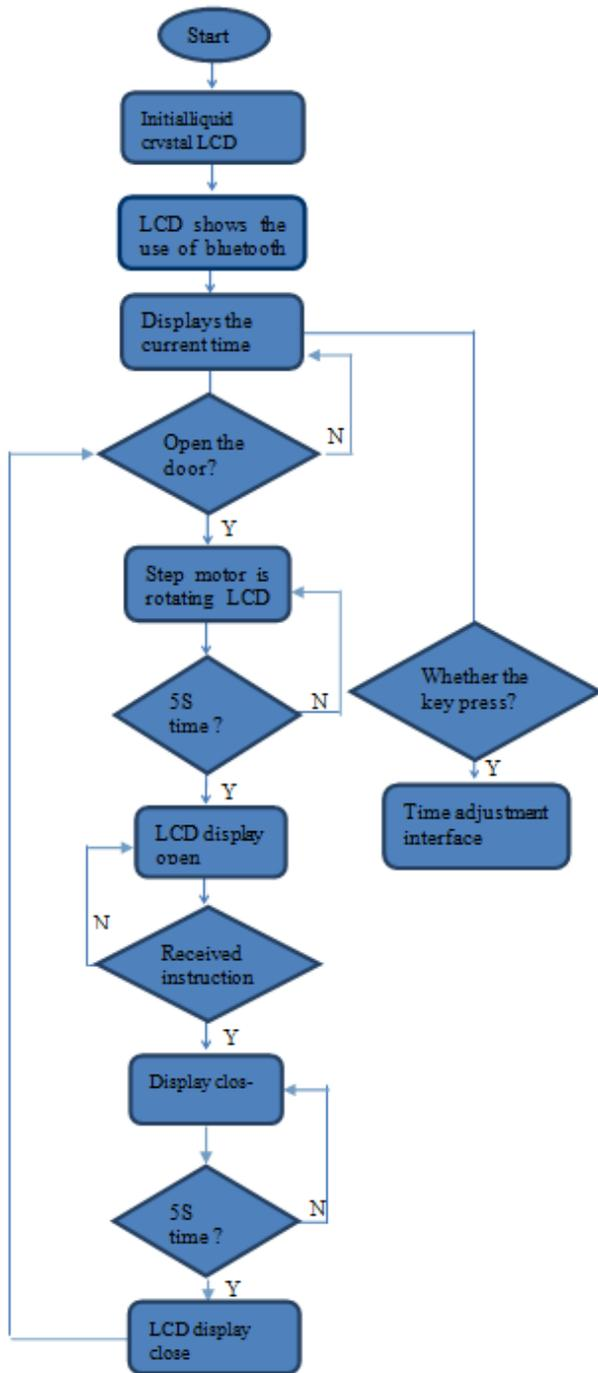
Fig. 7. Flow chart of software design
