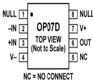
Figure 8 OP07 pinout
