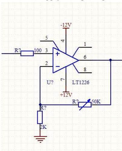
Figure 11: voltage amplifier module
