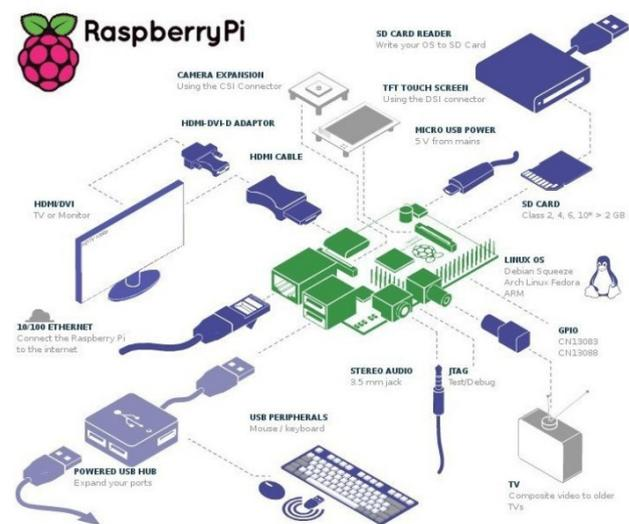
Fig 1 The macro-structure of the Raspberry Pi B plate
