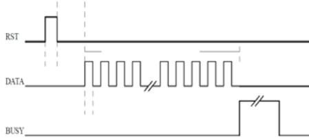
Fig 5 Serial Timing Diagram
