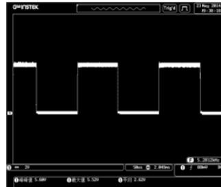
Figure B Peak value of pulse voltage for 20V
