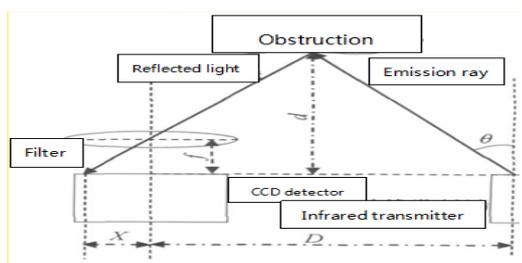
Fig.1.1 The principle diagram of the triangulation ranging
