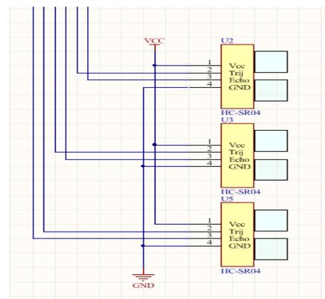
Fig 4 ultrasonic transceiver circuit
