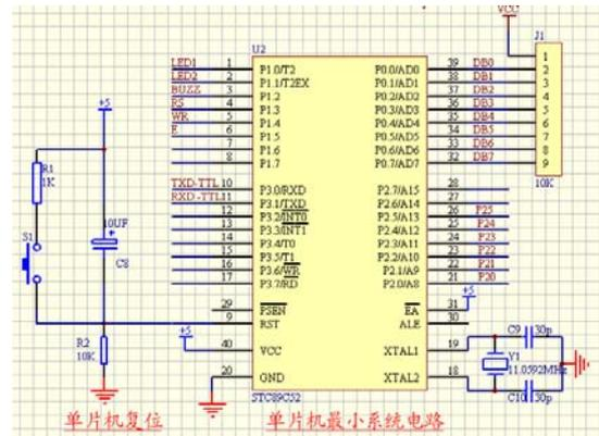
Fig. 2. Circuit connection diagram with LCD12864
