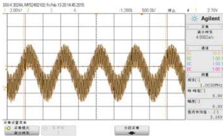
Figure 20 1MHz sine wave
