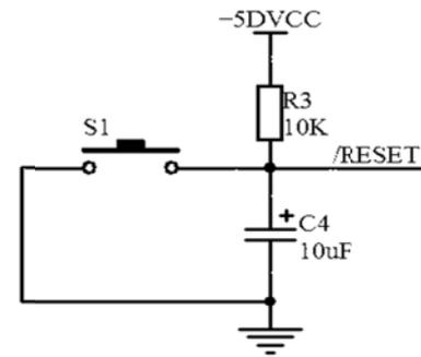
Figure 5 Reset circuit
